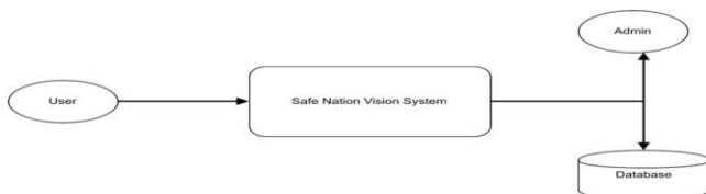
Fig. 3. Data flow diagram, Level 0 (context diagram).
