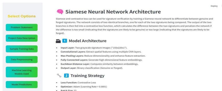
Fig.13. Siamese Neural Network for Signature Verification using CNN and Contrastive Loss
