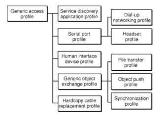
Service discovery application profile describes how an application should use the SDP (described in "The Bluetooth Protocol Stack") to discover services on a remote device. As required by the GAP, any Bluetooth device should be able to connect to any other Bluetooth device. Based on this, the service discovery application profile requires that any application be able to find out what services are available on any Bluetooth device it connects to.
