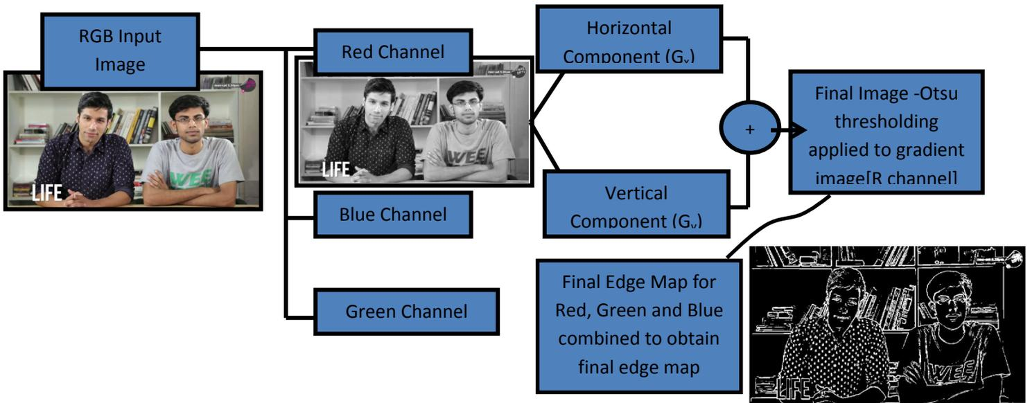
Figure 1: Graphical flow chart of the Sobel Edge detection algorithm implemented
