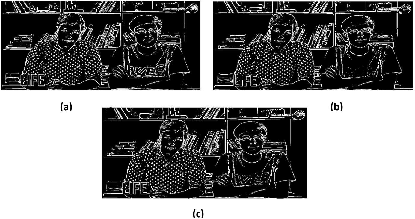
Figure 6: Edge Map of the Image for the (a) Red (b) Green and (c) Blue Channel
