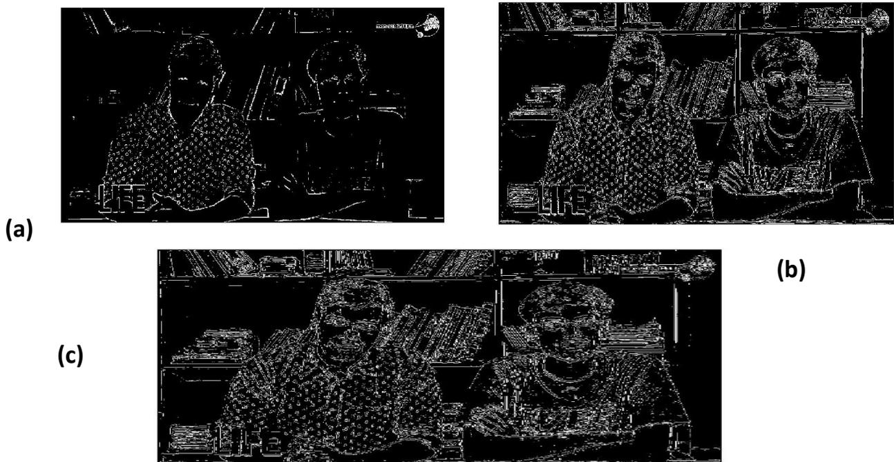
Figure 7: Marr Hildrith Edge Map of the Image for (a) N=3, sigma=0.6 (b) N=7, sigma=1 (c) N=17. Sigma=1.4
